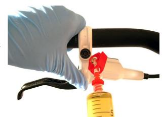
10 Stop pushing on the plunger of the calliper syringe. Unscrew the calliper syringe from the calliper or close the calliper bleed nipple and disconnect the bleed tube. For callipers fitted with a bleed port screw allow a small bead of brake fluid to form inside the bleed port and then refit the bleed port screw. Torque to 1.3-1.5Nm. **Do not over tighten.**
