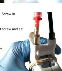
**6** Gently pull on the plunger of the calliper syringe to create a vacuum within the calliper. This will release any air bubbles which may be trapped inside the calliper.
