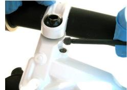
4 Remove the lever bleed port screw using the Torx screwdriver bit and set aside safely. Screw in the syringe and threaded bleed adaptor. Close the tube clamp on the syringe tubing.
