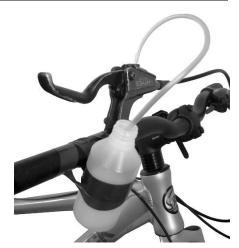
NOTE: If you leave your wheel and pads in situ, wrap a cloth around your calliper to protect your disc and pads from fluid spillages.
